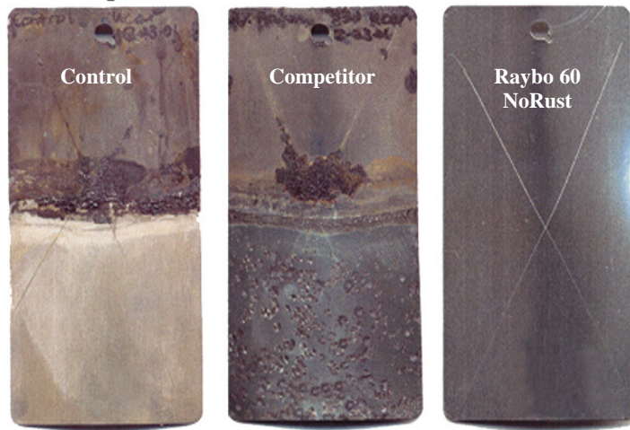
Panels partially immersed in UCAR 379 for 23 days (49°C, pH adjusted to 9.0)
